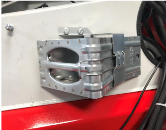
Wheel chock for safe parking of the machine
