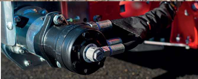
Belt drive is via hydraulic motor OMR with leakage oil line - a coupling for tension-free drive sits in between.
