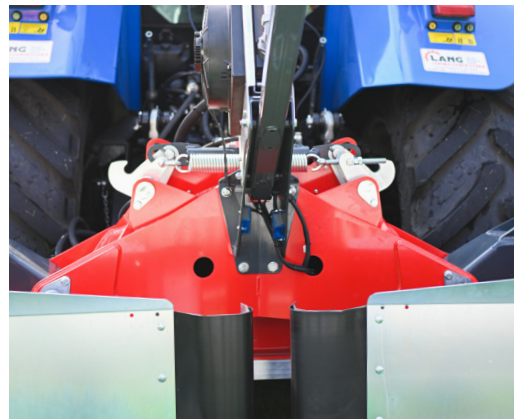
Mechanical transport lock of the outriggers
